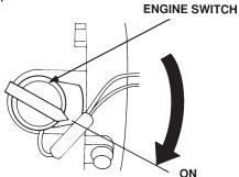
Figure 10. Engine ON/OFF Switch (ON Position)
