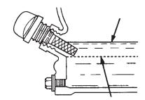
Figure 5. Engine Oil Dipstick (Oil Level)
