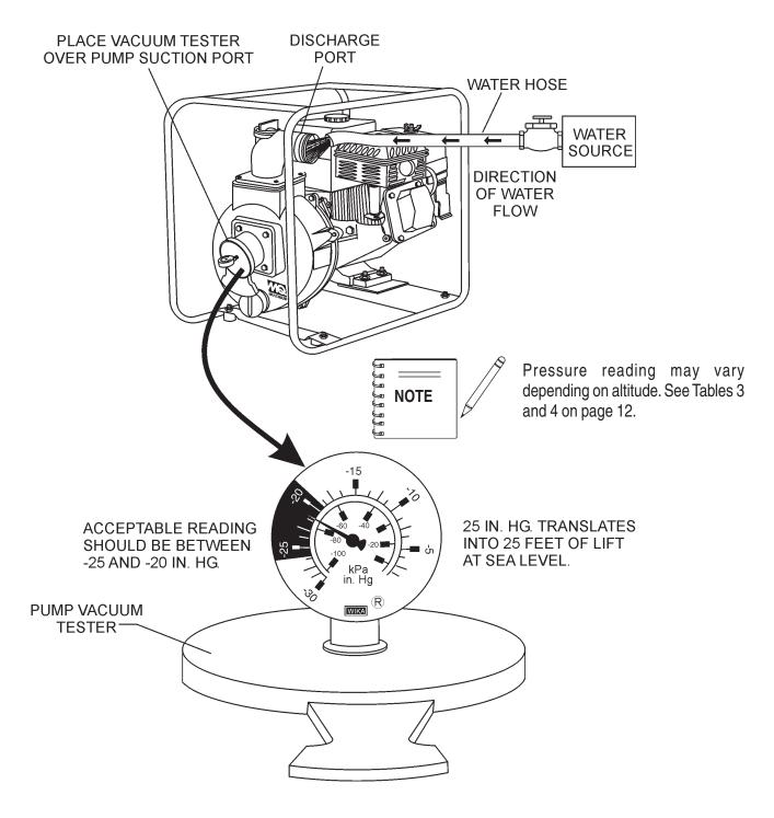
Figure 17. Pump Vacuum Tester
