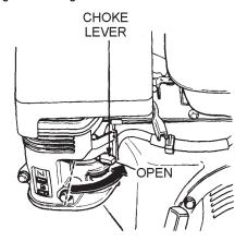
Figure 8. Engine Choke Lever (Open)
