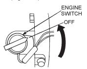
Figure 15. Engine ON/OFF Switch (OFF)
