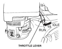
Figure 7. Throttle Lever (1/3 Start Position)
