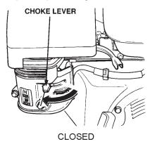
Figure 12. Choke Lever (Closed)
