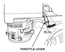
Figure 13. Throttle Lever (Run)
