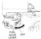
Figure 16. Fuel Valve Lever (OFF)
