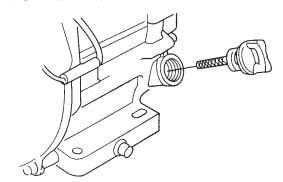
Figure 4. Engine Oil Dipstick (Removal)
