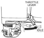
Figure 14. Throttle Lever (Idle)
