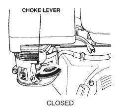
Figure 9. Engine Choke Lever (Closed)
