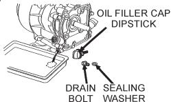
Figure 19. Engine Oil (Draining)
